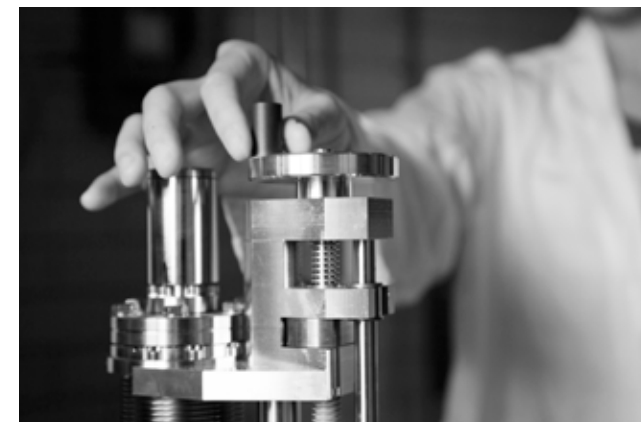
The components pictured, part of OCCAM's new x-ray photoelectron spectrometer (Thermo Scientific EscaLab 250Xi), allows for in-vacuo sequestering of samples, as well as transfer of samples between orthogonally oriented vacuum chambers.
