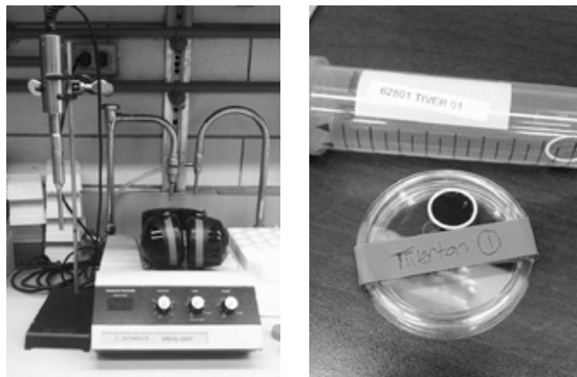
Jandi Kim and team used the titanium probe sonicator to extract particles loaded on the Tapered Element Oscillating Microbalance (TEOM) Filter.
